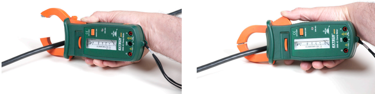
Figure 7 — Using clamp-on ammeter
