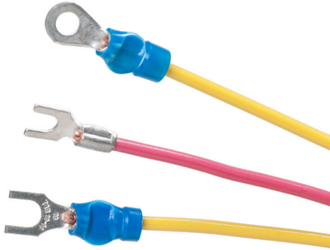
Figure 15—One-part crimp-on connectors
