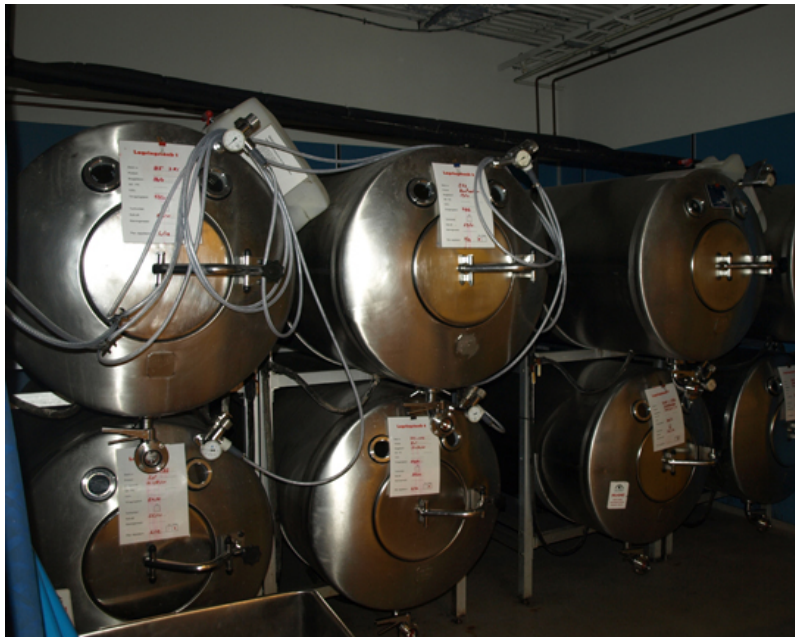
Figure 4.22 Fermentation of grape juice to make wine produces \text{CO}_2 as a byproduct. Fermentation tanks have valves so that pressure inside the tanks can be released.
