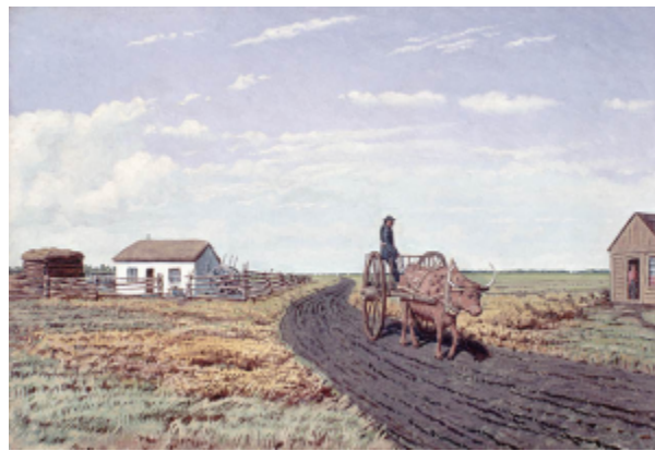
Figure 8.18 Red River carts were amphibious craft consisting of a flatbed attached to two large, convex spoked wheels. No metal was used in their construction and the wheels could be removed and strapped to the bottom so that the vehicle became a raft. They were invariably pulled by oxen. (Painting by William Hind, c. 1862)
