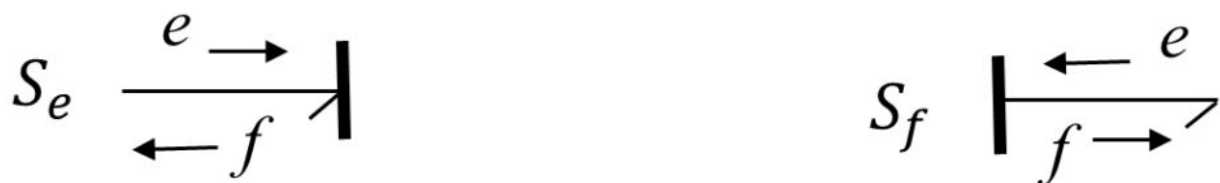
Figure 3-12 BG symbols for effort source (left) and flow source (right) with their assigned causalities
