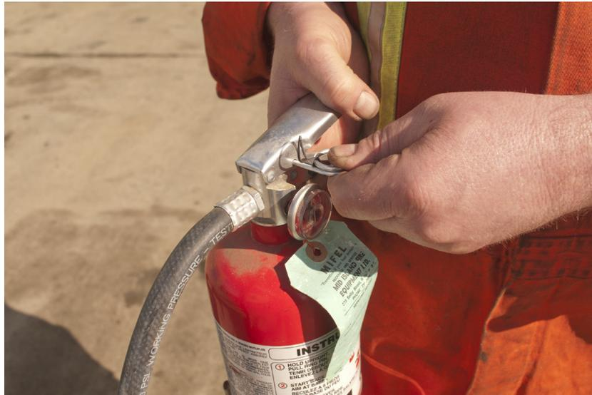
Figure 1 — Pull the pin
