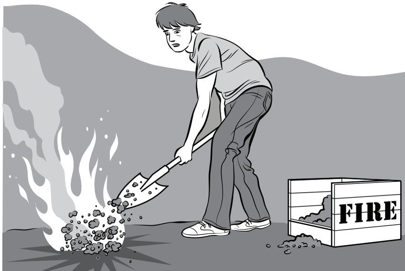
Figure 3 — Extinguishing powder applied by shovel or scoop
