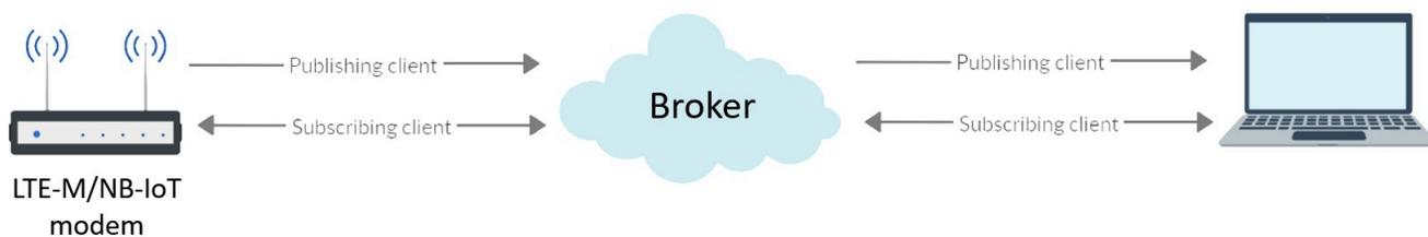
Figure 4.1. MQTT protocol for cellular IoT
