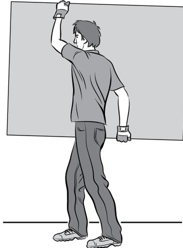
Figure 1 — Carrying a large sheet of a panel product
