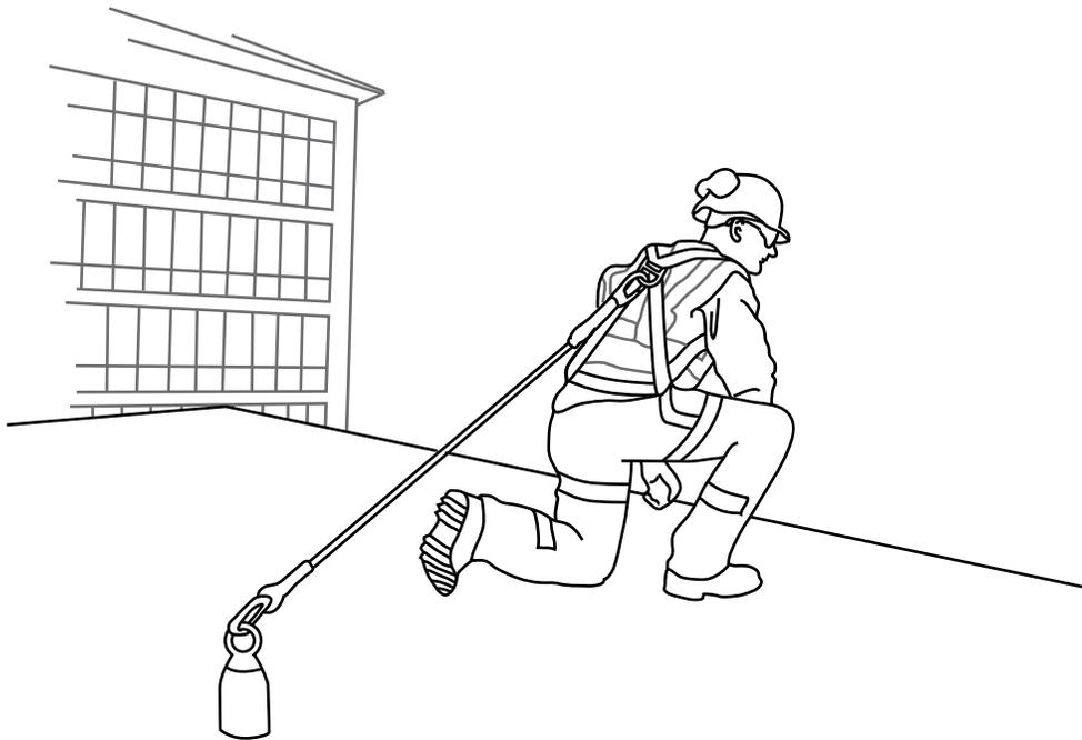
Figure 1 — Fall restraint
