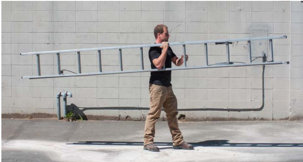
Figure 2 — Lifting a ladder
