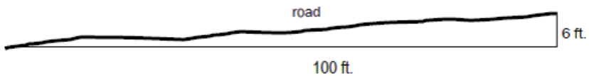
Figure 1.3. A road climbs at a gradient of 6%. The road gains 6 feet in elevation for every 100 feet of horizontal distance. Note that the length of the road itself is longer than 100 feet.
