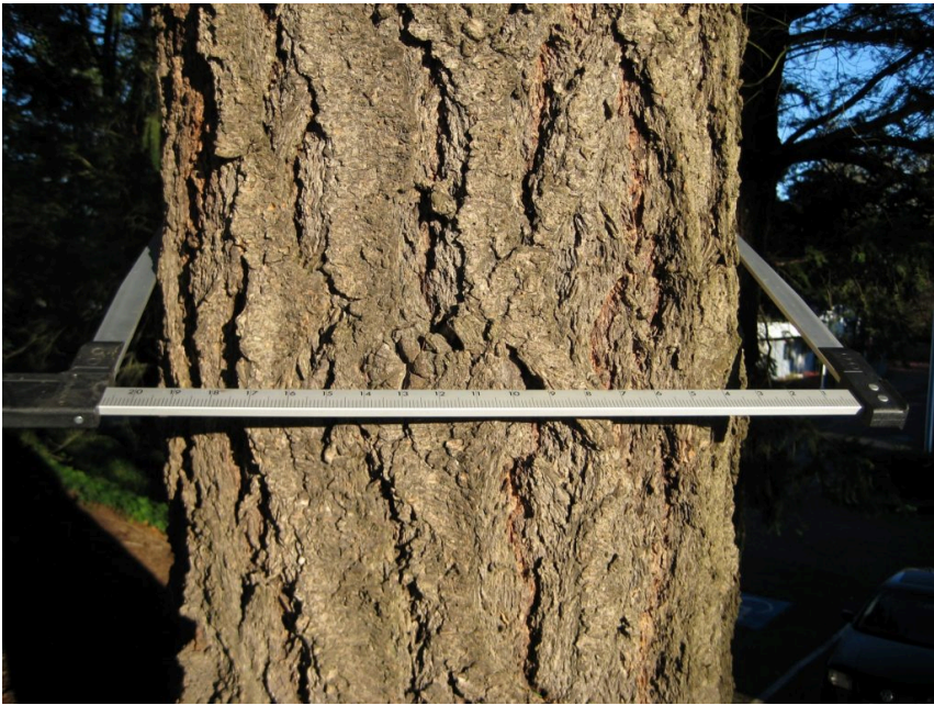
Figure 3.13. A tree caliper is held at right angles to the tree trunk. Diameter is read off the left side of the sliding scale at front.
