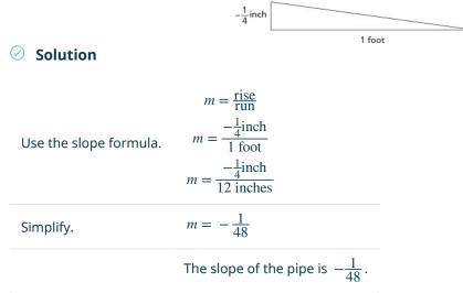
The pipe drops 1 inch for every 48 inches of horizontal run.
