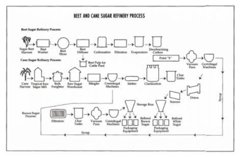
Figure 2. Sugar refining process.
