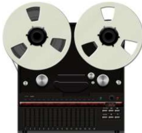
*Reel-to-reel tape recorders and magnetic tape not only helped artists experiment with overdubbing, but they also were a compact method for reproducing and preserving audio.*
