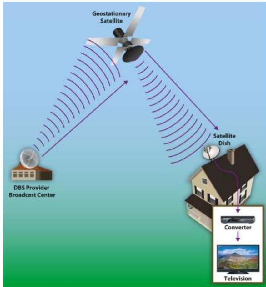
*Subscribers of DBS receive signals from geostationary satellites that are broadcast in digital format at microwave frequency and intercepted by a satellite dish. A converter next to the television produces output that can be viewed on the television receiver.*
