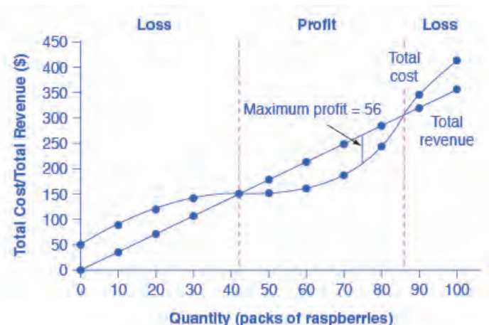
Figure 8.2 Total Cost and Total Revenue at the Raspberry Farm Total revenue for a perfectly competitive firm is a straight line sloping up. The slope is equal to the price of the good. Total cost also slopes up, but with some curvature. At higher levels of output, total cost begins to slope upward more steeply because of diminishing marginal returns. The maximum profit will occur at the quantity where the gap of total revenue over total cost is largest.
