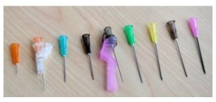
Variety of needles with different gauges and lengths. Note only two of these have safety system technology as part of their structure.
