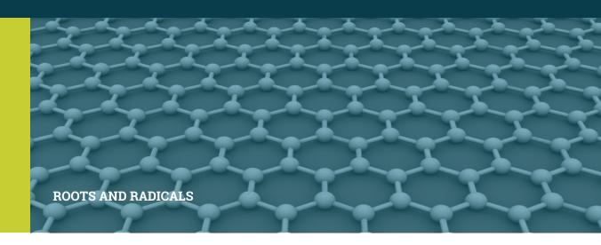
**Figure 8.1** Graphene is an incredibly strong and flexible material made from carbon. It can also conduct electricity. Notice the hexagonal grid pattern. (credit: "AlexanderAIUS" / Wikimedia Commons)
