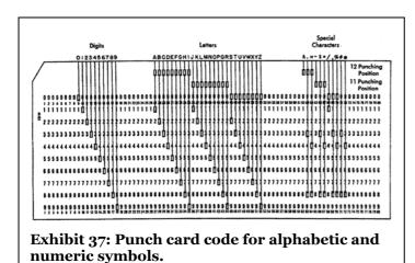
Punch card storage was not very dense by today's standards. The cards measured 3 ½ by 7 3/8 inches, <sup>22</sup> and a deck of 1,000 was about a foot long. Assuming that all 80 columns are fully utilized, that works out to about 48,000 characters per cubic foot, which sounds good until we compare it to PC thumb drives which currently hold up to 8 billion characters.
