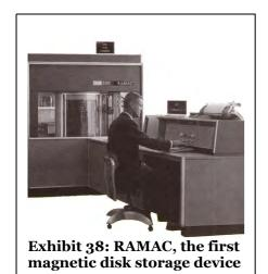
IBM shipped the RAMAC on September 13, 1956. The disk could store 5 million characters (7 bits each) using both sides of 50 two-foot-diameter disks. Monthly rental started at USD 2,875 (USD 3,200 if you wanted a printer) or
