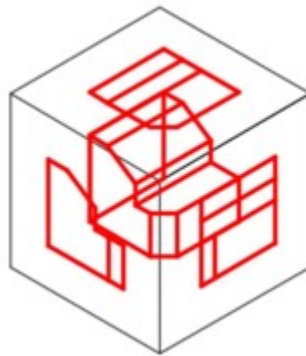
Figure 8-3 The Glass Box Principle
