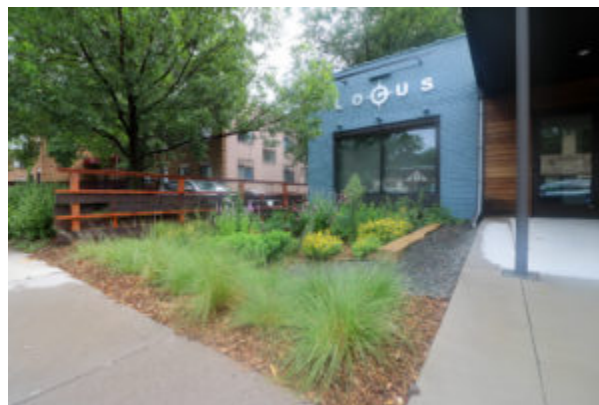
Figure 9.4 Example of a rain garden
