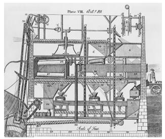
**Figure 9.5** Oliver Evans was an American engineer and inventor, best known for developing ways to automate the flour milling process, which is illustrated here in a drawing from a 1785 instructional book called *The Young Mill-Wright & Miller's Guide*.
